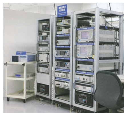
Power Calibration System
